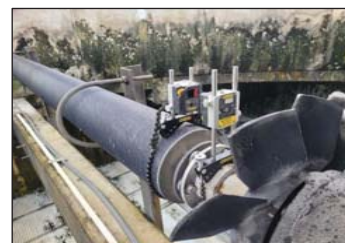
Pict. 7 Adjust drive shaft alignment gearbox after.
